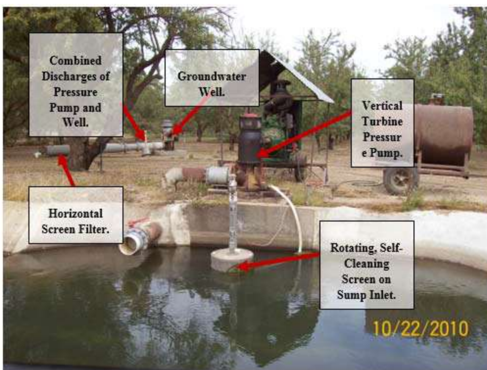
Figure 6-9 Rotating, Self-Cleaning Screen Filter Followed by Vertical Turbine Pressure Pump and Horizontal Screen Filter for Almond Irrigation. Screen Filter Installed Downstream of Combined Discharges of Pressure Pump and Groundwater Well
